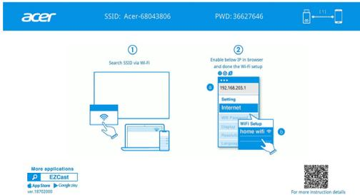
2. After successful connection, the IP address will appear on ② and the SSID will disappear on ①.
