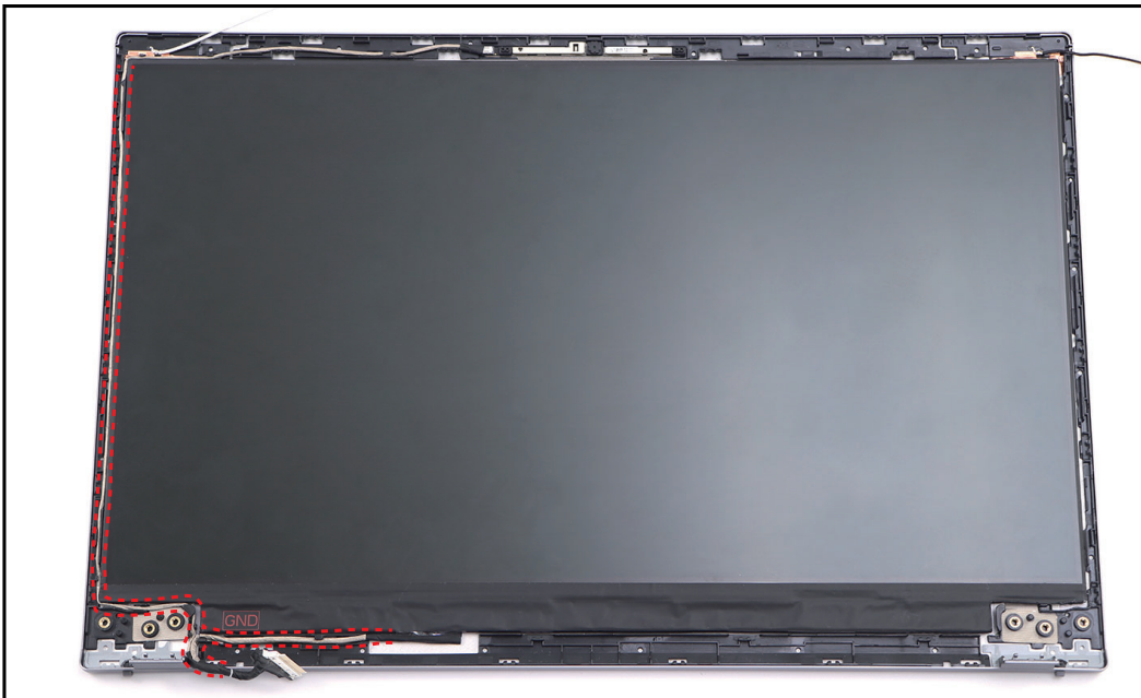
Figure 1-48. Unrouting the eDP Cable
