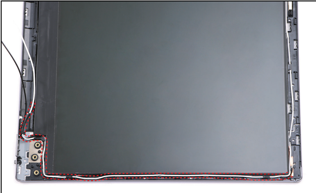
Figure 1-45. Unrouting the Auxiliary Antenna Cable
