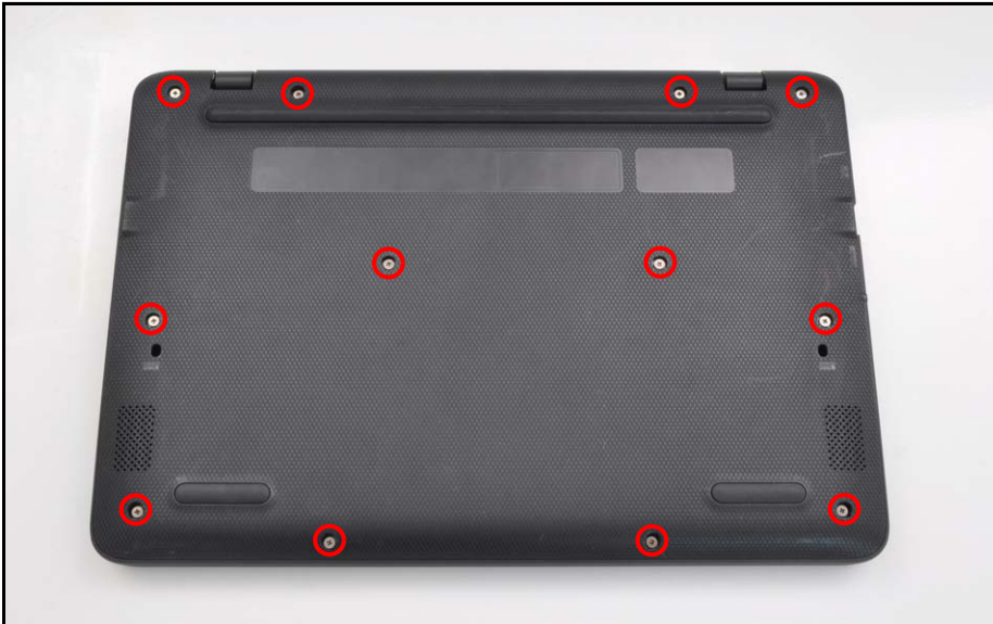
Figure 1-3. Base Cover Screw Location
