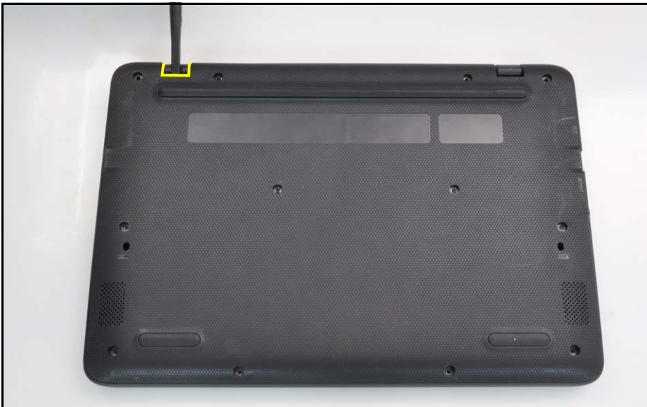
Figure 1-4. Base Cover Removal
