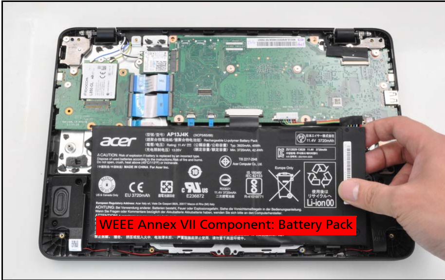
Figure 1-9. Battery Pack Removal
