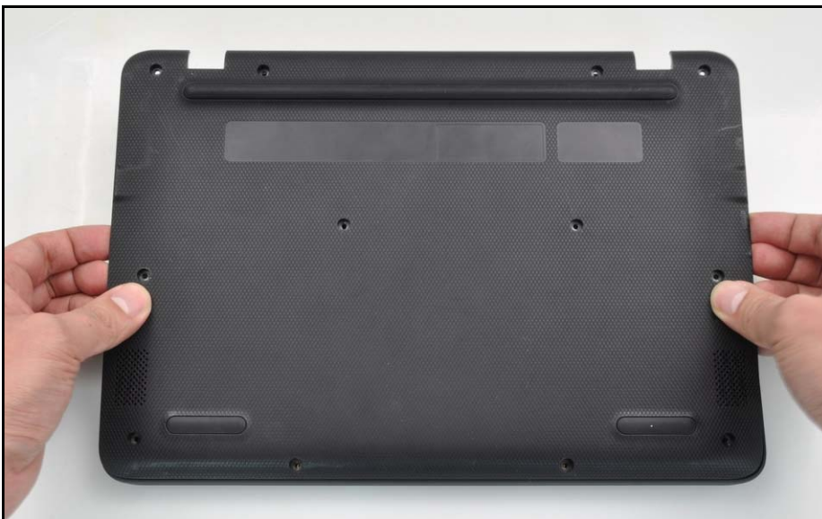
Figure 1-6. Base Cover Removal
