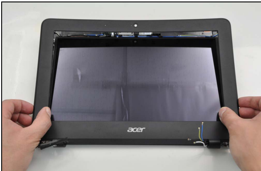
Figure 1-33. LCD Bezel Removal
