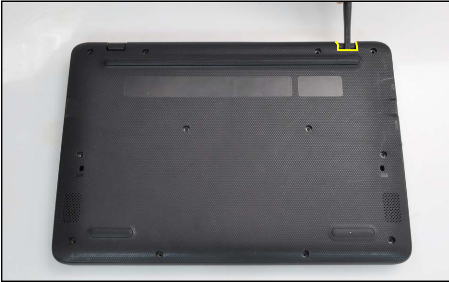
Figure 1-5. Base Cover Removal
