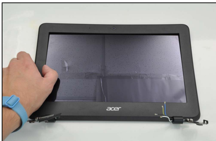
Figure 1-31. LCD Bezel Removal
