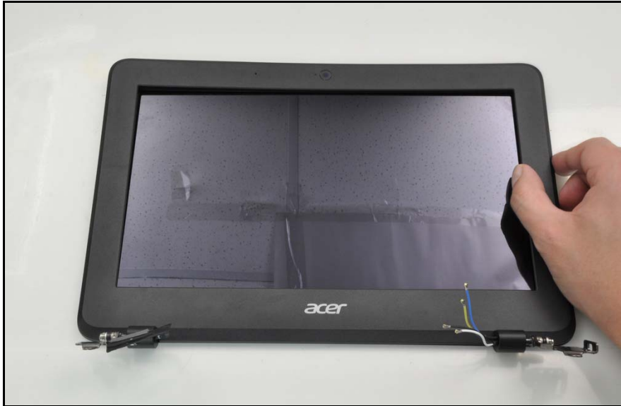
Figure 1-32. LCD Bezel Removal
