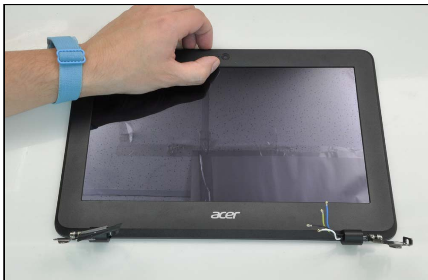
Figure 1-30. LCD Bezel Removal
