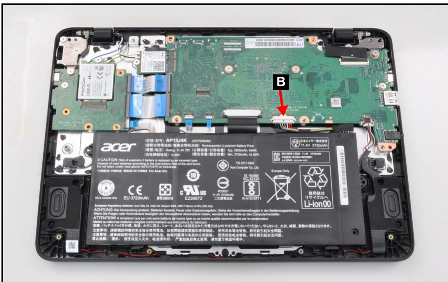
Figure 1-8. Battery Pack Removal
