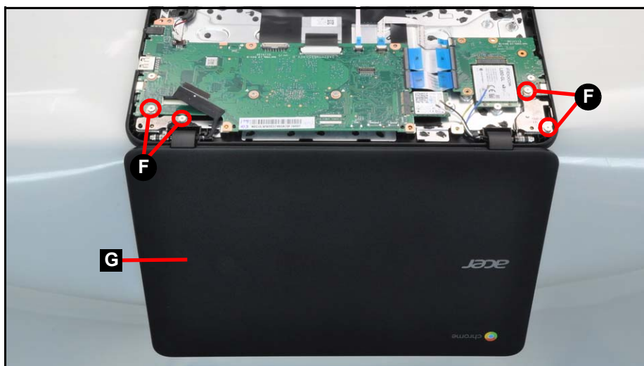
Figure 1-14. LCD Module Screw Location
