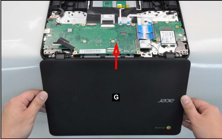
Figure 1-15. LCD Module Removal
