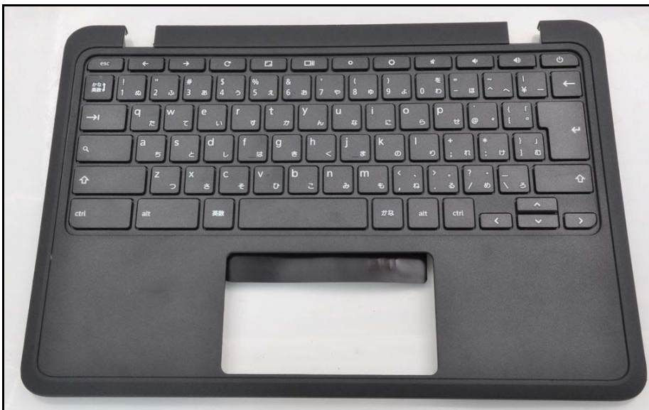
Figure 1-37. Top Assembly (Keyboard)
