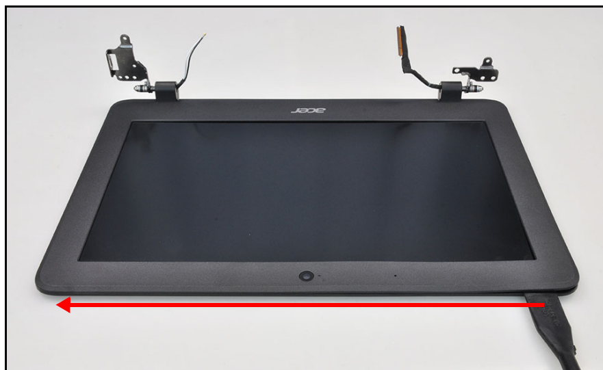
Figure 1-26. LCD Bezel Removal
