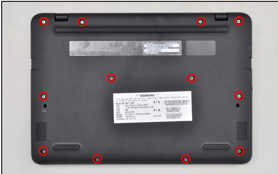
Figure 1-3. Base Cover Removal
