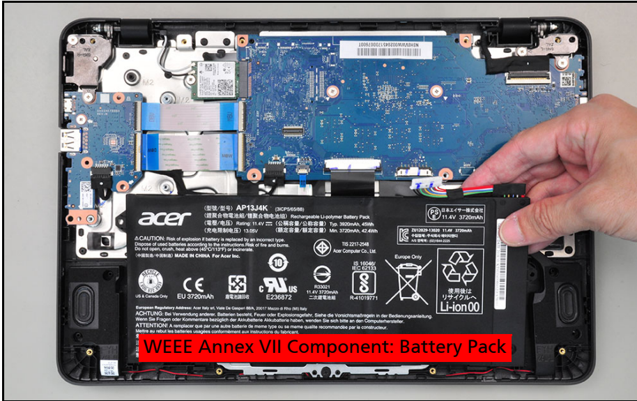
Figure 1-8. Battery Pack Removal
