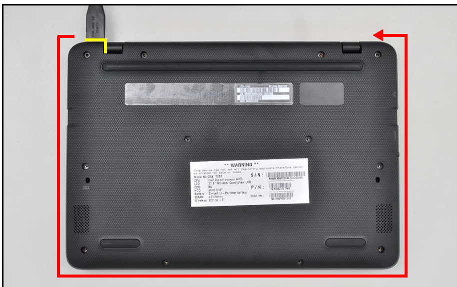
Figure 1-4. Base Cover Removal
