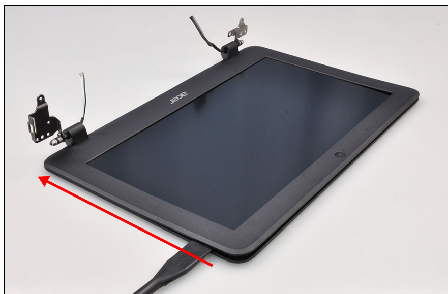
Figure 1-27. LCD Bezel Removal
