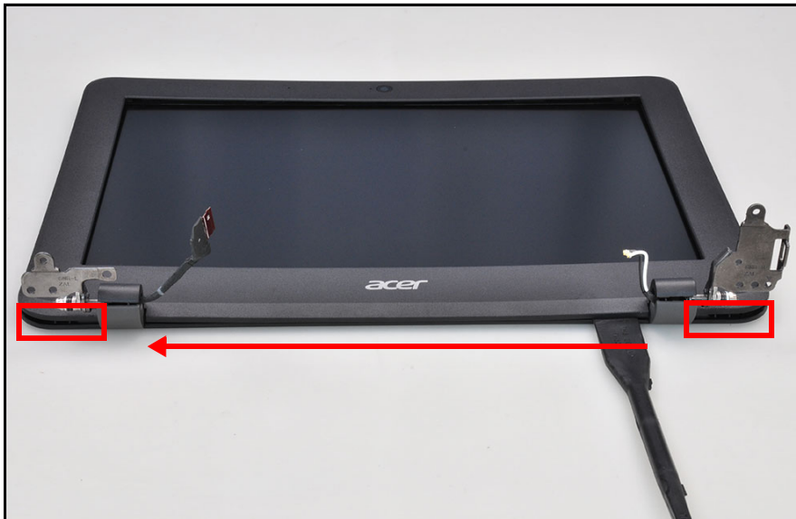
Figure 1-29. LCD Bezel Removal
