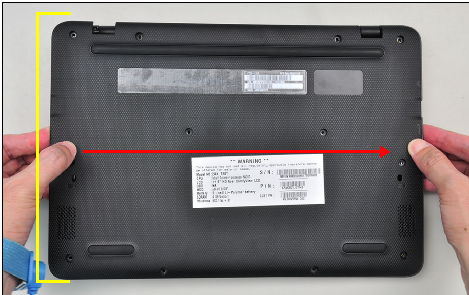
Figure 1-5. Base Cover Removal
