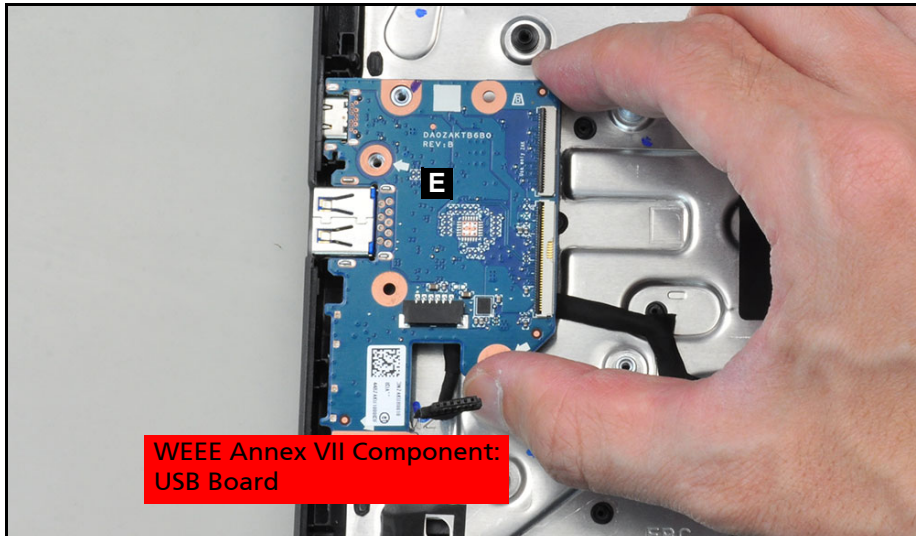
Figure 1-20. USB Board Removal
