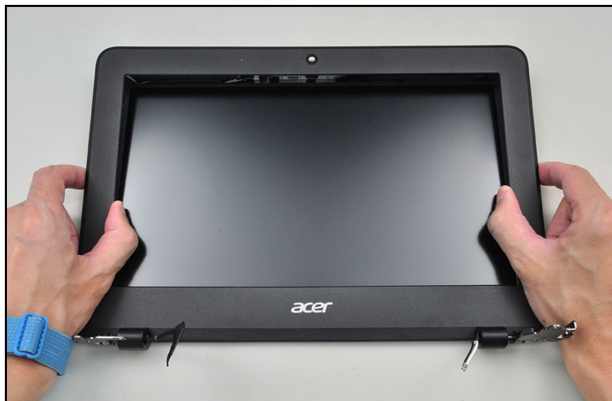
Figure 1-30. LCD Bezel Removal
