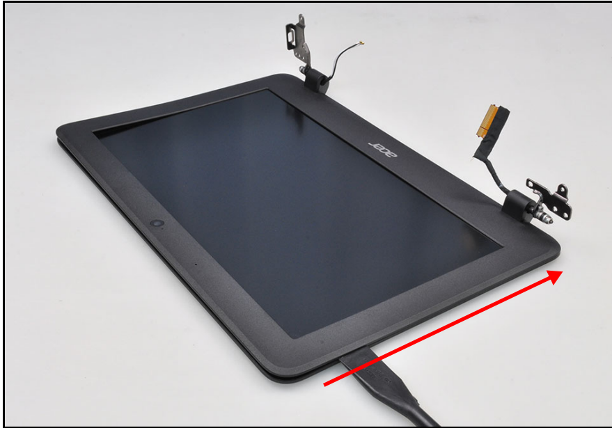
Figure 1-28. LCD Bezel Removal
