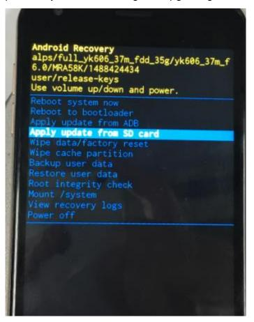
4) Then select the SW files, press power key to go on upgrading.
